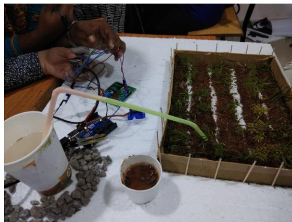
Figure6.6. model of Smart Irrigation System using IOT
